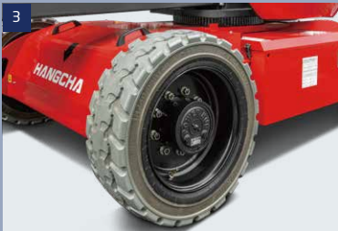
Tires: foam-filled tires with good off-road performance
